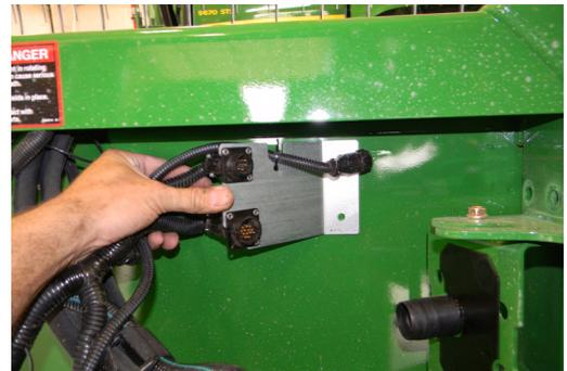
4. For "50 series" heads, Connect 204 to the 31p OEM connection mounted on the head.
