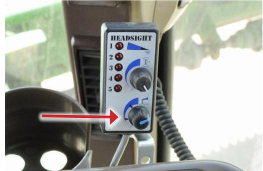
2. Because the Headsight box is designed to work with many OEM sensors, it may be possible for the operator to choose a height that is too low for proper operation, meaning the sensors would never send a raise signal.
