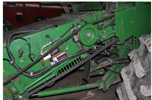
4. Zip tie harness to existing hydraulic hoses and wiring.
