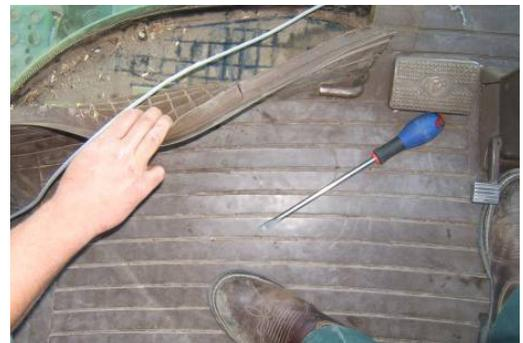
3. Route under ladder platform and following existing hydraulic hoses/electrical wiring on the left side of feederhouse.
